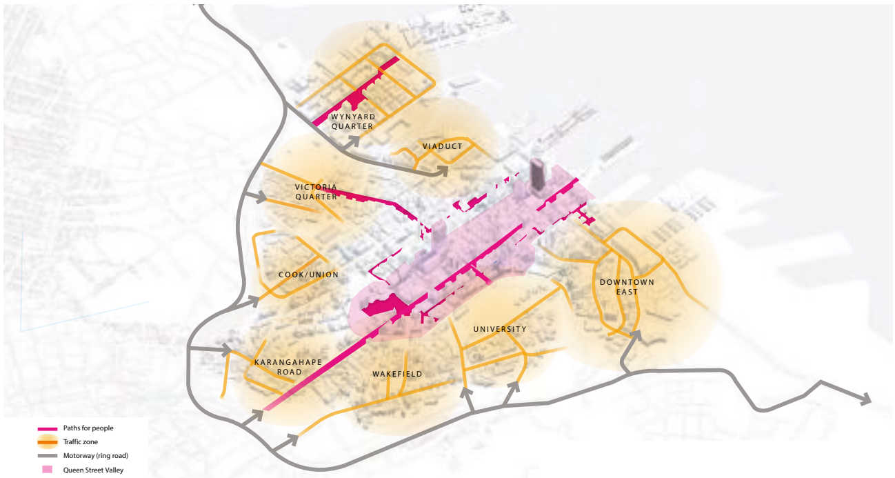
Access for Everyone (A4E) concept diagram: Auckland city centre with an indicative low-traffic neighbourhood surrounding a pedestrian-prioritized Queen Street Valley. Source: Access for Everyone
